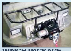
WINCH PACKAGE Warn winch with 2,500 lb. capacity and roller fairlead, 50 ft. of cable. (All vehicles)
