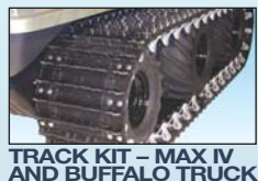
TRACK KIT - MAX IV AND BUFFALO TRUCK 1" deep lugs provide extra traction for the heavier loads carried by the MAX IV and Buffalo Truck. Lowers ground pressure to nearly one PSI with full load. Includes wheel extensions, outer bearing cages and frame rail for extra axle support. Requires 21" Goodyear Rawhide tires and solid axles.
