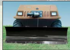
PLOW Steel blade. 5 swivel positions. Snow and light utility. Includes winch. 60" and 76" widths available. (Available on all models)
