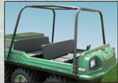
ROLL CAGE Black pipe 1-5/8" O.D., protects four people. Includes seat belts for four. (MAX IV)
