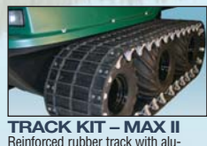
TRACK KIT - MAX II Reinforced rubber track with aluminum tire guides lowers ground pressure to less than one PSI, fully loaded. Turns MAX into a tracked vehicle for use all year round on snow, mud, and marsh. Kit includes wheel extensions, outer bearing cages and frame rail for extra axle support. Requires 21" Goodyear Rawhide tires and solid axles.
