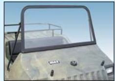
WINDSHIELD Aluminum frame, safety glass. Folds down. (MAX II)
